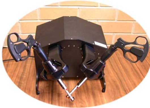
Figure 1. The input device is a Laparoscopic Surgical Workstation
